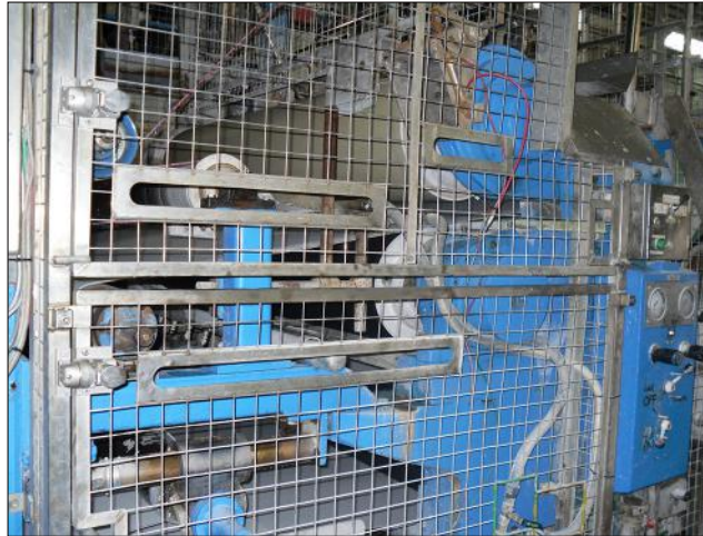
Figure 28 Press section enclosed with fixed guarding
