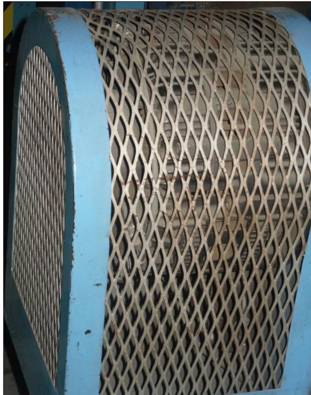
Figure 5 An example of a fixed guard to protect a rotating shaft
