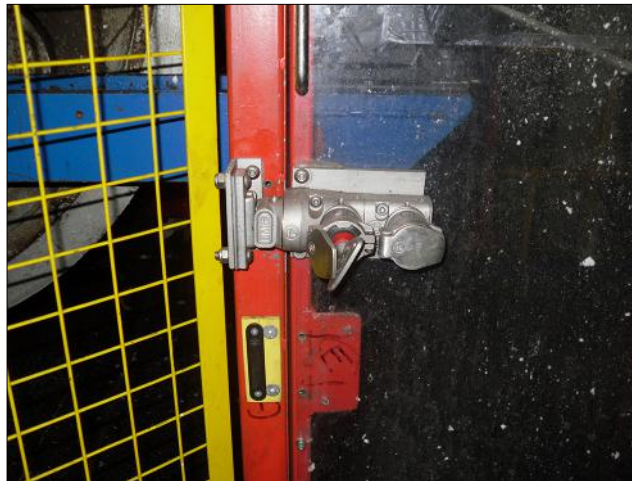
Figure 4 Example of an interlocked guard with trapped key
