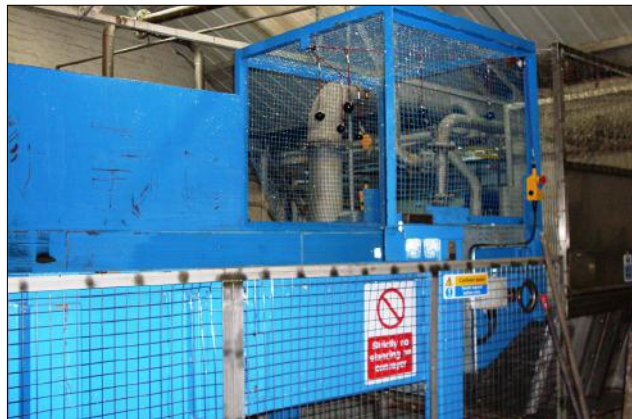
Figure 16 An example of a horizontal conveyor feeding a pulp storage tank in the stock prep area using fixed guarding and extended sides
