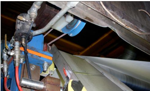
Figure 13 Examples of air feed chutes
