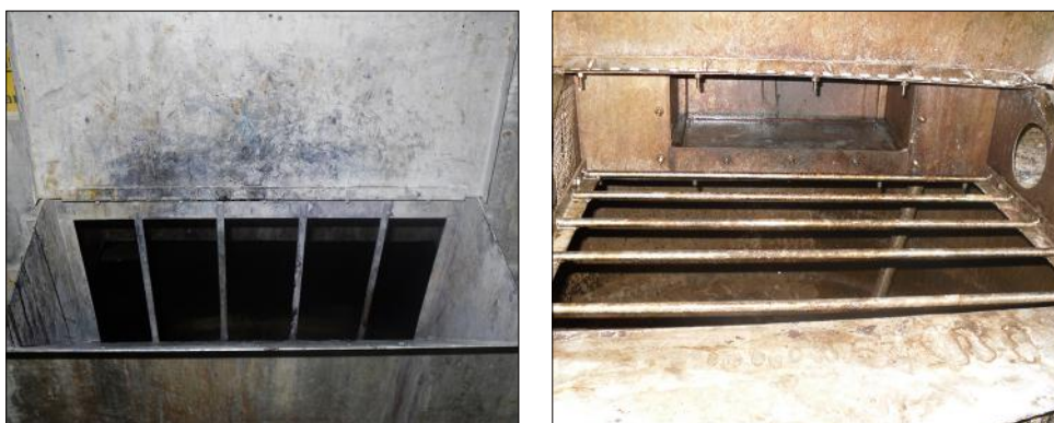
Figure 20 Example of fixed grilles on side and top openings of a pulper. Both fixed grilles have been added to prevent whole body access
