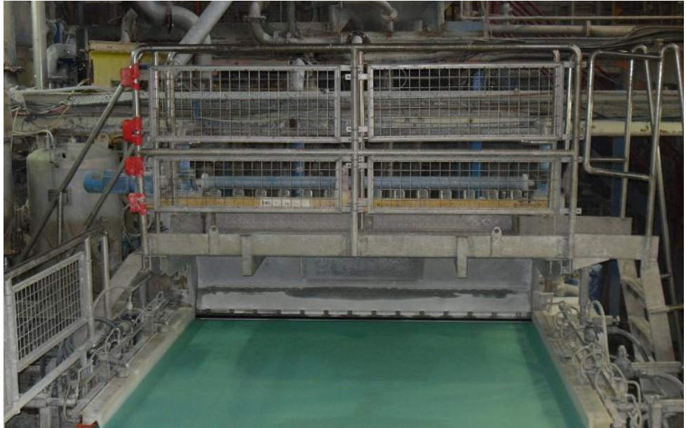
Figure 26 Protective structures and railings used to prevent access to the wire
