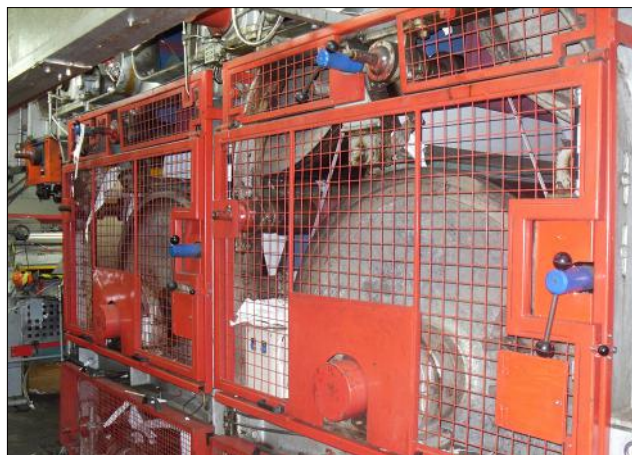
Figure 2 Example of fixed guarding in place to prevent access to the drying cylinders on a paper machine
