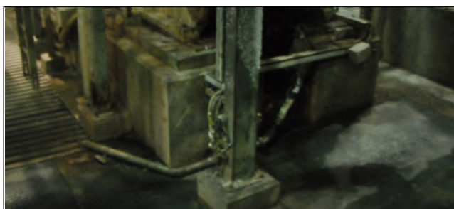
Figure 24 Contamination around the refiner being discharged into drains, cleaning will also be needed
